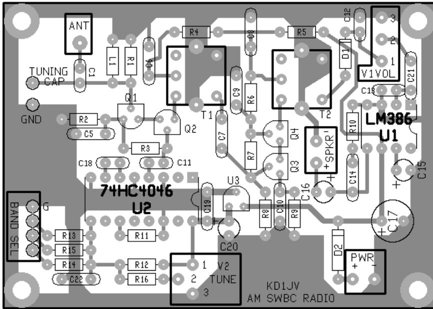
DRILL OVER SIZED HOLE OR COUNTER SINK FOIL TO ISOLATE PIN FROM GROUND
