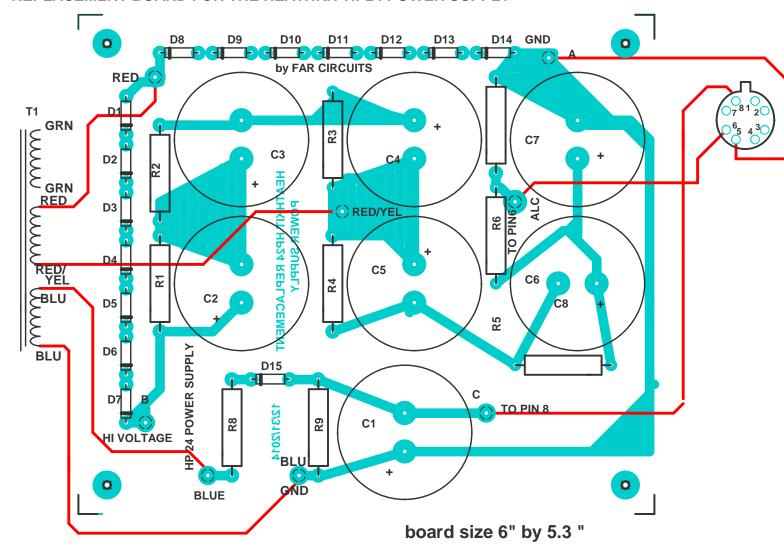
THIS ONLY SHOWS THE WIRING TO AND FROM THE P C BOARD, ALL OTHER WIRING REMAINS THE SAME
