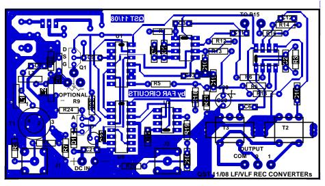
THIS IS THE CORRECT OOVERLAY FOR THE I/Q DETECTOR BOARD 7/27/09 DUPLICATE PARTS AND POLARITY OD D1 HAS BEEN CORRECTED.
