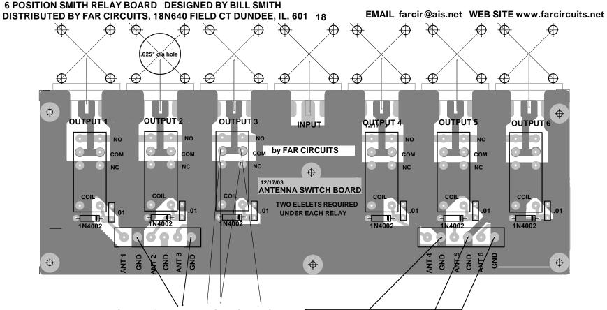
EYELETS ARE REQUIRED AT THESE LOCATIOMS UNDER EACH RELAY AND THE CONNECTORS, TOTAL 32 EYELETS ENCLOSED
