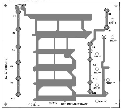
The circled areas in BLACK require eyelets. Insert the eyelet from the top side of the board and solder the rim of the eyelets and solder to the foil.
